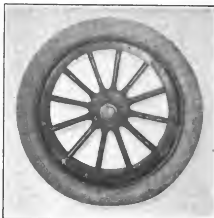
Fig. 6—Lambert remountable rim which is controlled by a single bolt
